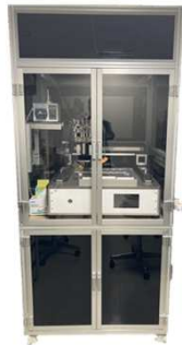
: Food Printer for making steak-type (Coaxial, Bench-Scale)
